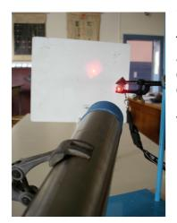
Then, just speak (it is better using a deep voice), make a sound (for example, with musical instruments like djembes, flutes, etc...) or place a radio in front of the other end of the pipe.
